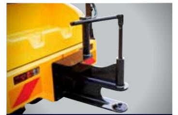
**Towing coupler with releasing lever (OPT)**
