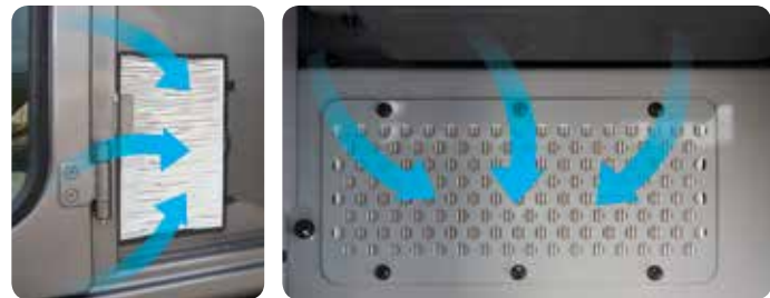
Cabin Air Fresh Filter The internal pressure is maintained to be slightly higher than that of outside to exclude dust and to reduce noise levels.
