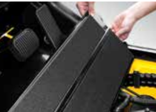
Tool-less floor plate for serviceability.
