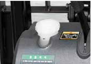
Brake fluid reservoir with level switch When brake oil level becomes lower than Min. the warning lamp on the cluster lights on.
