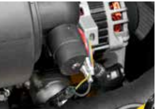
Electrically monitored air filter Air cleaner sensor alerts the operator of a restricted air filter and allows replacement before damage.
