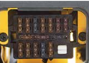
An accessible, compact fuse box for easy inspection
