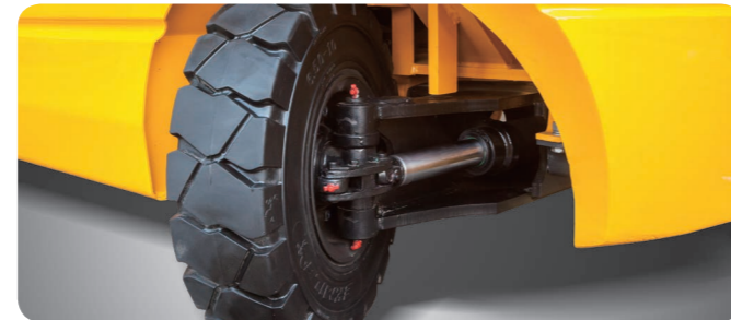
Fully hydrostatic power steering The hydraulic steering system always guarantees smooth and flexible steering, preventing over-run and kick-back.
