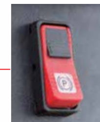
Parking Brake Switch With auto parking function when the operator is not in the seat
