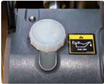
Brake Fluid Reservoir with Level Switch When brake oil level become lower than Min. the warning lamp on the cluster lights on.
