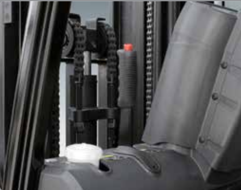
Parking Brake Ratchet type parking brake requires less effort from the operator to set.
