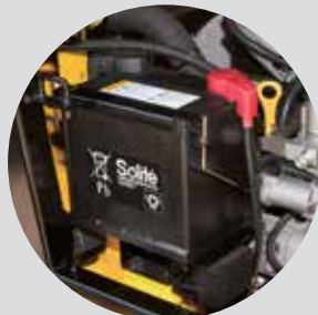
Rotational Battery Installation
