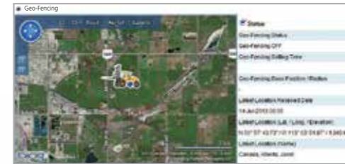
Hi-mate (Remote Management System) Hi-mate, Hyundai's proprietary remote management system, provides operators and dealer service personnel access to vital service and diagnostic information on the machine from any computer with internet access.
