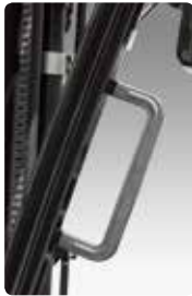
Large Footboard & Hand Grip Wide "open" step offers convenience and safety when entering and exiting truck.
