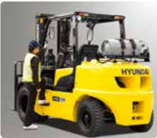
Large Footboard & Hand Grip Wide "open" step offers convenience and safety when entering and exiting truck.
