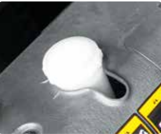
Brake Fluid Reservoir with Level Switch When brake oil level became lower than Min., the warning lamp on the cluster lights on.
