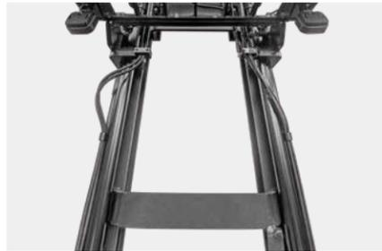
A new optimized lifting system enables the operator's wider view through the mast and excellent line of sight.
